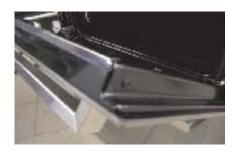
Remove screws from both side of door
